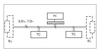
All units connected to the bus must have differing serial interface addresses (parameter 797).
