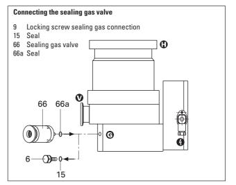
Please refer to Operating Instructions PM 800 229 BN for details on installing the sealing gas valve and adjusting the sealing gas flow.
